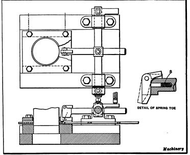
Fig. 36. Spring Toe Latch Stop
